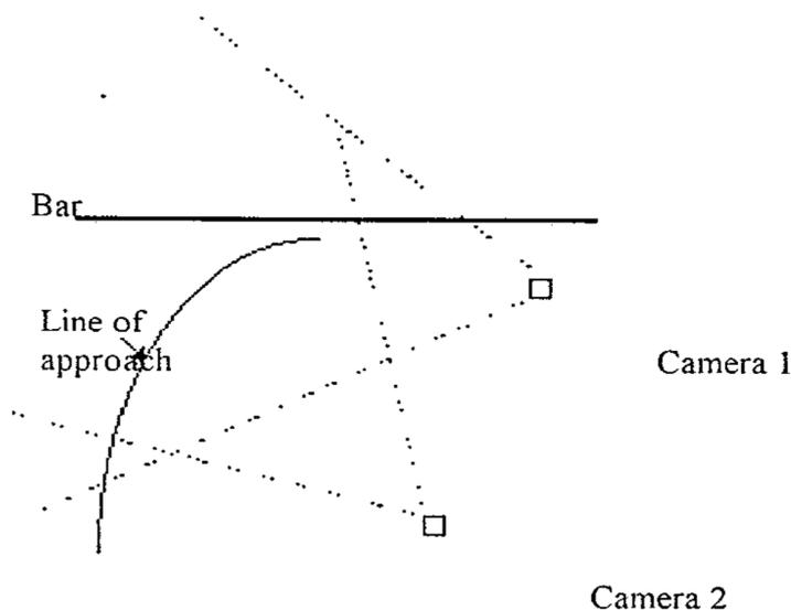
Figure 1: Arrangement and placement of two cameras
